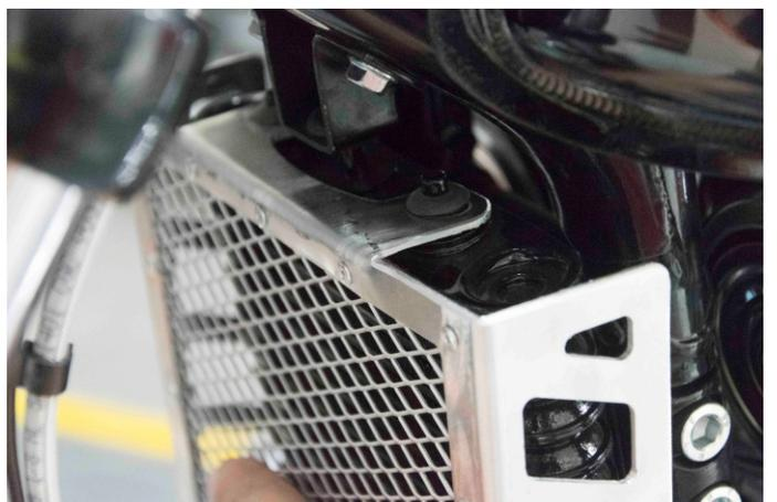
Place the rubbers that you will find in the installation package as shown in photo 3 and in the same way place the new radiator grill in its position.
