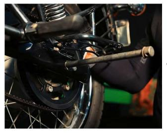
Insert the rear axle bolt through the swing arm holes, sleeves (spacers), wheel hub, and brake caliper. Do not tighten the bolt until the chain/belt tensioner(slider) is aligned.
