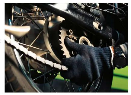
Now remove rear sprocket and hub with chain from wheel assy as shown.
