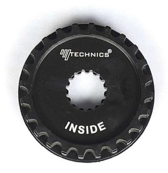
when installing the front conversion pulley, make sure the print 'inside' area faces towards the engine case and the flange area faces outward.
