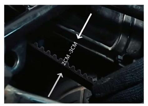
Do not over-tighten or loosen the belt. Check belt tension at every 3000 km.
