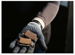
Before removing the rear axle bolt remove the brake pads by pushing out the pad locator pin
