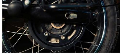
Insert the sleeve(spacer) on the left and right of the rear wheel hub then install the complete wheel assembly between the swing arm as shown above figure.
