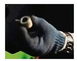
Remove and secure both left and right wheel spacers with a different dimension.
