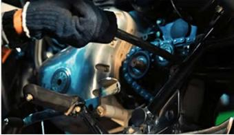
Remove the swing arm front end bolt 22mm and nut 24mm by using socket and secure the dust boot cover on both sides.
