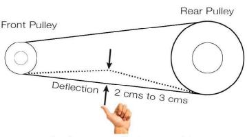
To check the belt deflection, you may do it manually by pushing on the middle of the lower belt towards the swing arm, while pushing the belt, permissible deflection is 2cms to 3cms. (the vehicle must be on the service/center stand or have no load at the rear axle)
