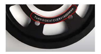
This figure shows the print on rear pulley(sprocket) as a reminder TURN SIDE AT EVERY 15000Kms.
