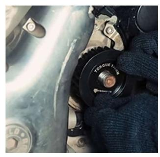
Now insert the front belt pulley (sprocket) and lock washer on the output shaft respectively
