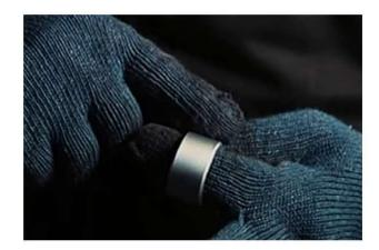
Clean the surface of the output shaft (front sprocket) and insert the short sleeve(spacer) supplied by Mtechnics conversion.
