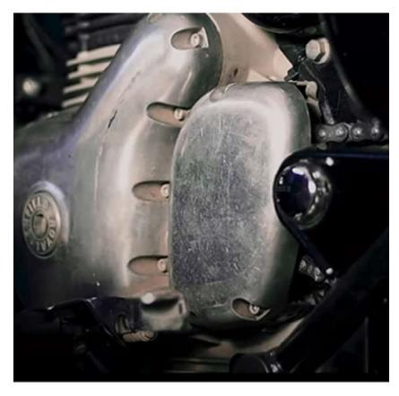
Remove front sprocket protection cover by using 5mm allen key.
