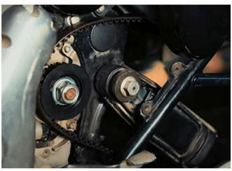
Mount back the swing arm assembly after cleaning the surface. Tighten the front long bolt and nut also the rear left and right shock absorbers lower end bolts. Follow the tightening torque by RE specified.
