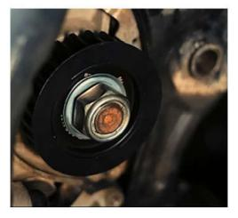
Remove the rear sprocket from the hub. Clean the hub surface.
