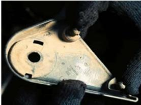
Unclip the cover and remove 10mm screw from both sides and pull out the decorative strip gently. Make sure the two legs insert are not broken as shown above.
