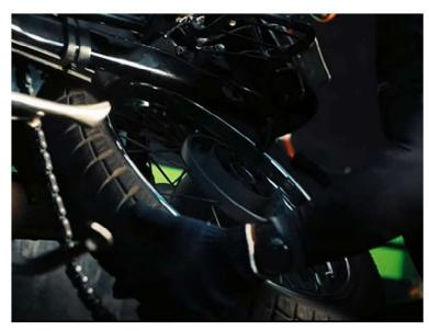
Remove the entire rear wheel assy out from the vehicle.
