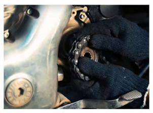
Pull out the front sprocket then the chain is free to remove out as shown in the above figure.
