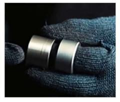
Pull out the stock sleeve(spacer) behind the sprocket as shown in the figure
