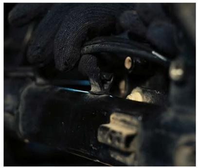
Unclip the cables of rear caliper and wheel speed sensor gently from swing arm.
