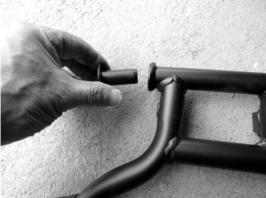
3. Grease the pivot pin and slide through the mounting points on the frame and through stand bushes
