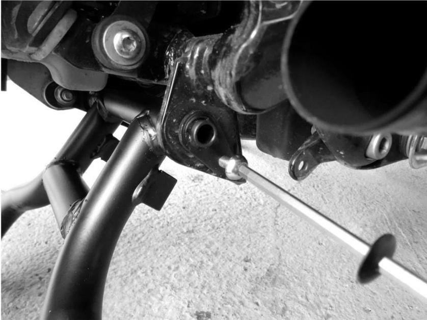
5. Fit the spring pivot screw to the frame after removing the plastic hole plug
