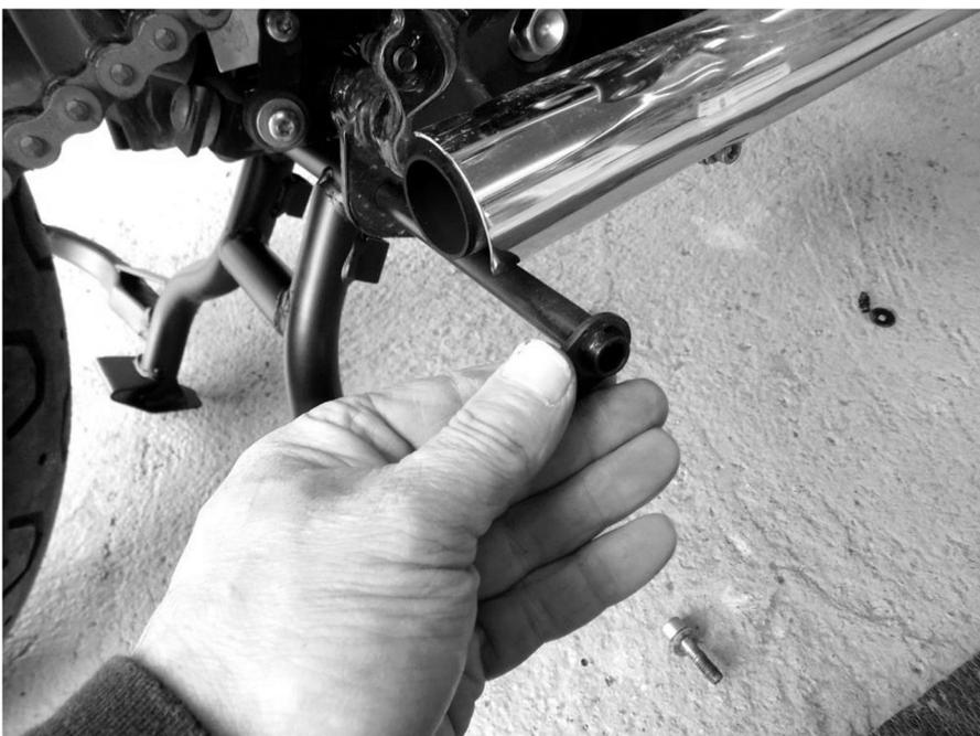
4. Locate bush with slipped button head bolt
