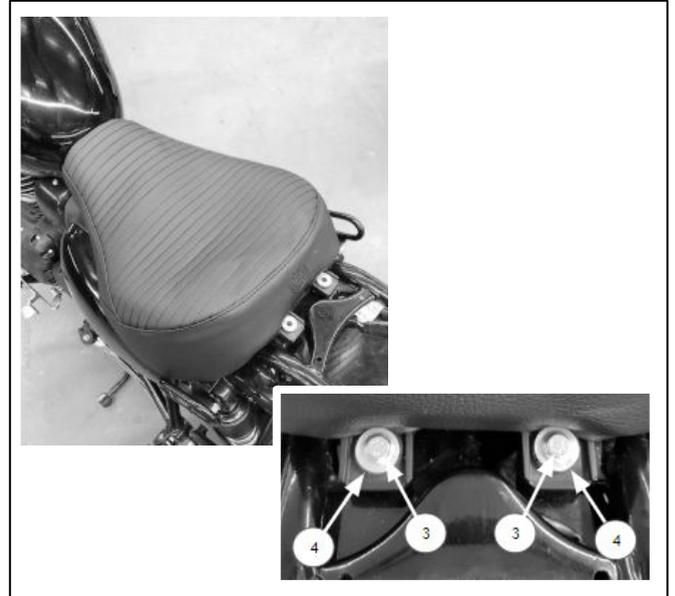
**7** Hook the passenger seat into the frame at the rear and align the front mounting holes. Ensure that all cords are tucked away under the seat and reinsert the bolt (1) through the grabrail boss and into the frame. Repeat for the other side of the vehicle. Tighten the bolts to **25Nm**.
