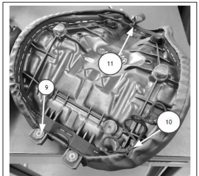
**6** Locate the front of the rider's seat onto the tab behind the fuel tank and align the rear mounting points with their corresponding holes on the frame. Reinsert the two sleeves (4) and two bolts (3) and tighten to **12Nm**.
