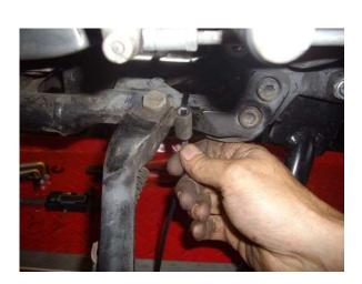
6. Check clearance to tyre (runs close on one side this is normal) and chain and lubricate pivots with spray grease (chain lubricant works well).
