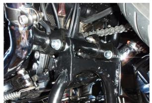
3. Fit 10mm bolt and spacer to 1/hand mount and tighten both the left and right-hand stand pivot bolts <u>firmly but not securely</u>. At this stage, the stand should be free on its pivots, if the stand is binding then one of the top-hat bearings will require spacing out from the frame, slacken the left-hand bolt, if the stand stops binding then remove bolt and fit packing washer behind top-hat bearing, this should alleviate the issue, retighten all bolts.
