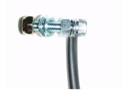
2. Test fit domed headed 10mm bolt and spacer with collar to right-hand stand hole as shown below. (Head of bolt must be to outside of bike or it will foul spring). With bolt ready to fit, hook spring to stand and pull-down stand to push through bolt, fit washer and nut LOOSELY at this stage! Note that both stand lugs go to right side of frame lugs. (Note added as many bikes are not like this arrangement).
