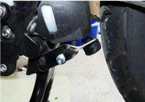
On T100 and Street Twin models with standard silencers fitted, apply some liquid soap or silicone spray to the stop rubber and fit into the hole provided in the Left silencer.
