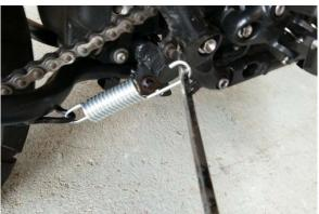
Fix the pivot pin with the locating screw using Loctite on the threads.
